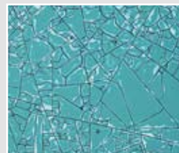
Stress cracks in acrylate layer Brightfield ACHROPLAN 10x/0.25
